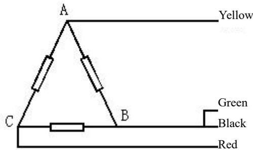
Wiring diagram in case of measuring ab and bc
