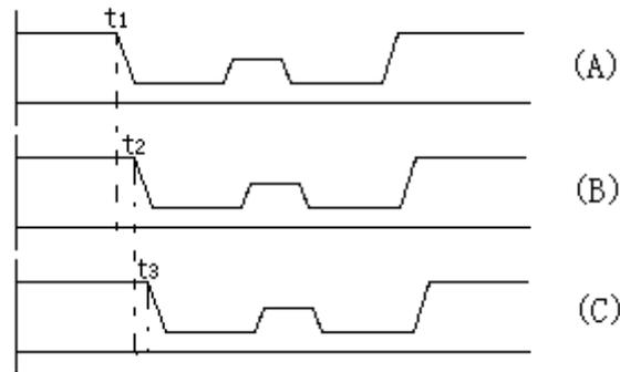
Figure 11 Non-simultaneous three-phase waveforms (assuming that phase A is ahead of phase B, and phase B is ahead of phase C)
