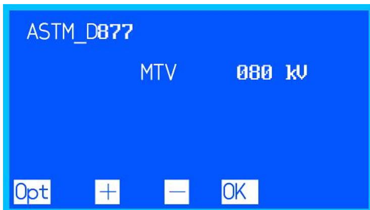
Picture 3 ASTM D877 MTV set up
