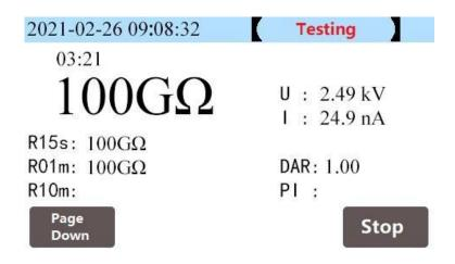
After starting the measurement, the instrument issues an audible and visual alarm and displays the measurement time. After the measurement, the instrument automatically depressurizes and discharges the test product, and displays the measurement data.
