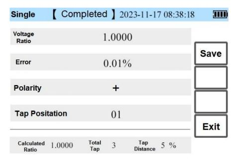
Touch the **Save** button to save the data, and press the "Test/Stop" button to retest.
