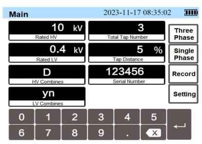
Rated HV: The rated voltage on the high voltage side of the tested transformer.
