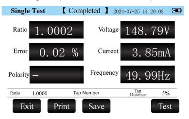
6.4 Three-phase transformer testing
